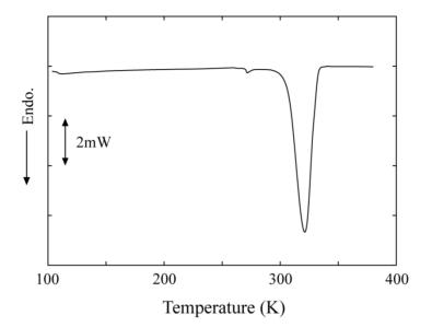
Figure 3. DSC curve for MDL-tartaric acid crystal on heating. The sample weight (powder) was 4.36 mg, and the heating rate was 5 K min<sup>-1</sup> under a dry N<sub>2</sub> gas flow of 40 ml min<sup>-1</sup>.
